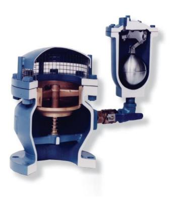
The Vacuum Breaker is designed to prevent vacuum conditions from occurring in pipes or tanks. After a power failure or rapid draining of the system, a vacuum condition often occurs in a pipe or tank. The pressure difference between the inside vacuum and outside air will cause a downward force on the float. At vacuum pressures greater than -0.25 psig, the float will compress the spring and move downward allowing free flow of outside air into the pipe or tank to eliminate the vacuum.
